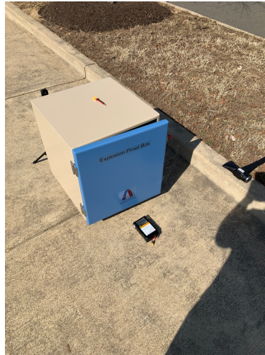
Figure 2.17: Battery test box.
