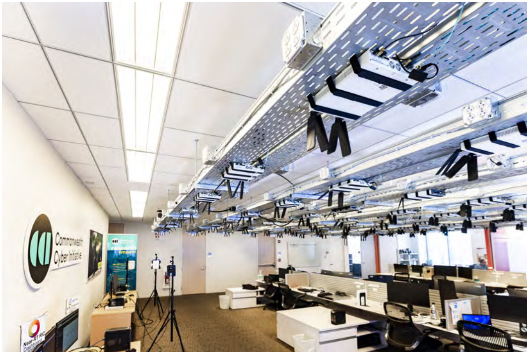
Figure 1.6: CCI xG testbed, indoors portion, in CCI Hub at VT.
