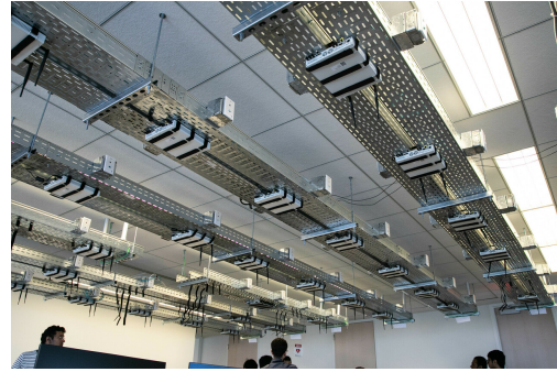
(b) xG testbed, with 72 latest generation software defined radios.
