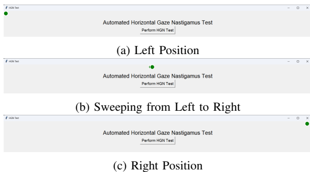
Fig. 3: Positions of the Dot During the HGN Test
